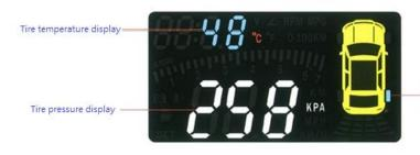
Tire pressure indicator light cycle Light indicates that the corresponding tire, tire pressure working properly
